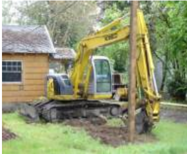
Figure 4-2. Track hoe equipment reduces soil compaction.
