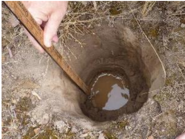
Figure C-2. A shovel was used to dig most of the way then a 6" diameter post hole digger was used to reach the proposed bottom elevation of a rain garden. Measure the drop in water from a known, stable marker.
