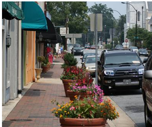
Figure 4-18. Contained planters are a common beautification project that benefit the watershed when placed over impervious surfaces. In a dense, “main street” application like this photo, the planter footprint shouldn’t exceed the width of the furnishing zone (i.e. the pavement area between the curb and the walking area of the sidewalk), which is the area where signs, benches, parking meters or other similar infrastructure might be placed. This will ensure that sidewalk traffic is not impeded by a narrowed throughway.
