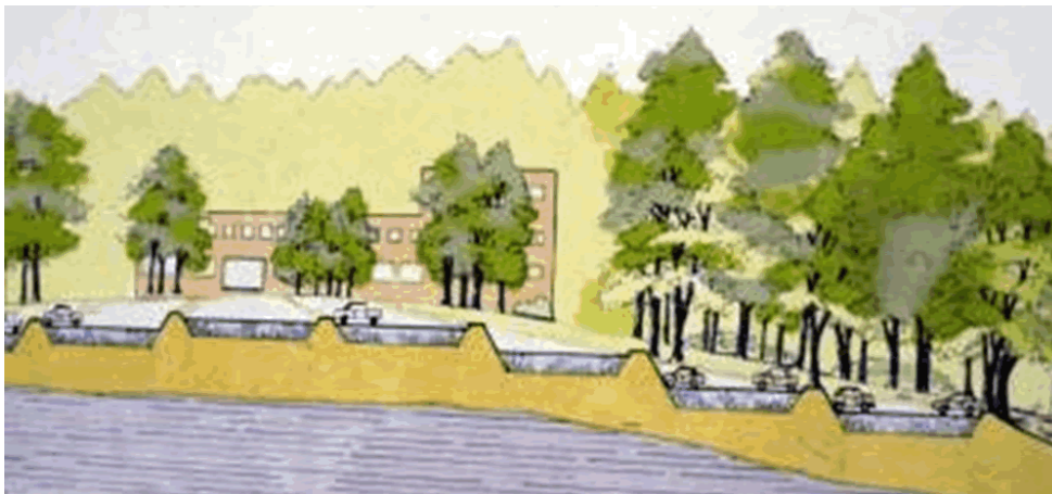
Figure 4-87. Soakage trenches below pavement are shown here. Stepping along existing contours reduces excavation and increases infiltration capacity. Graphic courtesy of Cahill & Associates.
