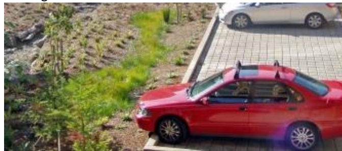
Figure 4-1. Site-scale treatment train. A rain garden (light green grassy area), porous pavement (parking lot), tree canopy, and native plants all work together to protect water resources, on and off site.
