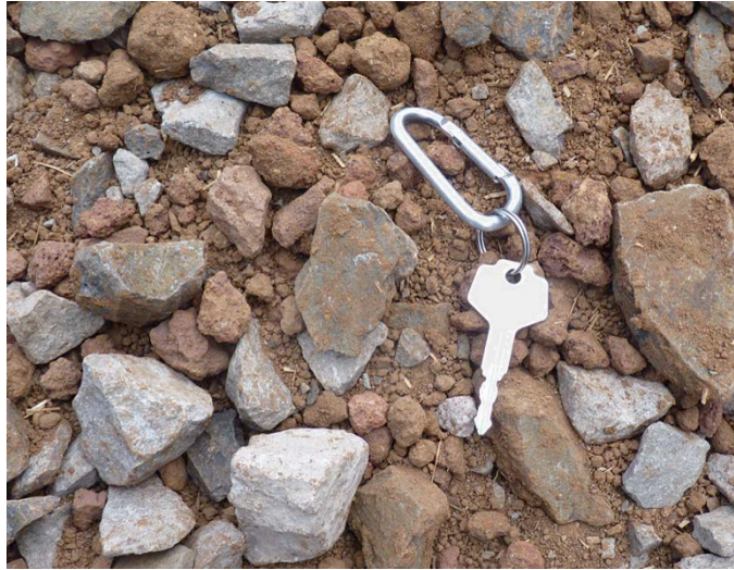
Figure 4-25. Structural soil is a blended soil mix of angular open-graded (i.e. all the same or similar size) rock, clay, stabilizer, and water that, when correctly and lightly compacted supports traffic loads and healthy tree root growth. The keychain is for scale.
