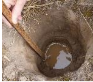
Figure 1-3. Infiltration testing identifies faster draining soil areas at the site scale (see Appendix C), regardless of soil type.
