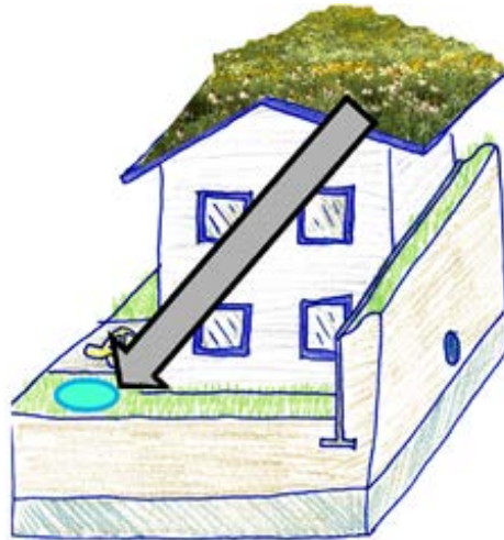
Figure 5-2. In this runoff reduction example, the vegetated roof is the only surface generating runoff, so this is directed to a rain garden. Other surfaces, per Figure 5-1, don't generate runoff (i.e. porous pavement) or are assumed to not generate runoff (i.e. restored soils). The approach for this site would satisfy the requirements of the LID Implementation Form.
