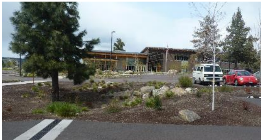
Figure 3-5. A meticulous grading plan and a willing contractor limited disturbance by protecting many existing trees in this newly developed parking lot.
