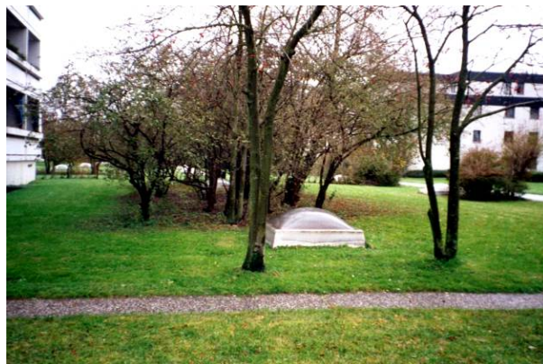
Figure 4-29. A vegetated roof above an underground parking facility serves as a park at the street level. Trees need three feet of soil and can add a lot of weight; however, one strategy for accommodating trees is to add soil depth and place trees only over building columns or load bearing walls.
