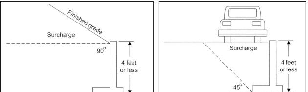
3) Wall less than 4' in height measured from the bottom of the footing to the highest point of any portion of the wall located within 45 degrees of an existing structure measured from the base of the wall to the bottom of the building footing. The Building Official and/or the City Engineer shall determine the extent of report needed.
